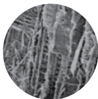
Cell structure – normal kiln dried timber
