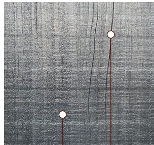
Laminated glue seams | Face check
