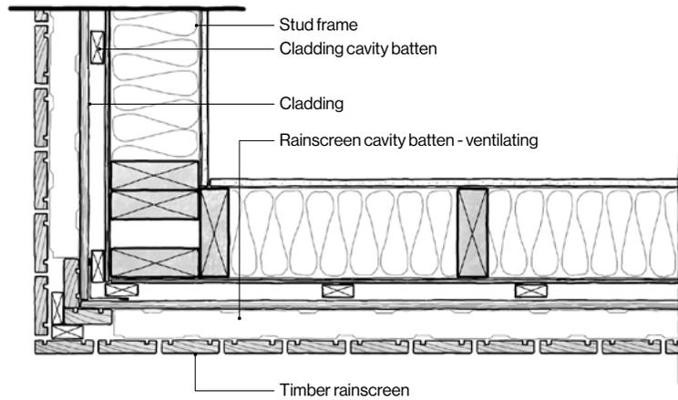
Sheet cladding such as plywood or fibre cement on cladding cavity batten with rainscreen cavity battens over top. Normally the cladding has a paint finish.
