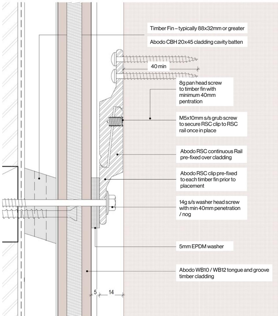
Abodo RSC batten clip system. Contact Abodo for further information.
