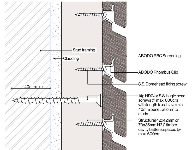
Abodo Rhombus Clip rain screen system. Refer Abodo Technical Data Sheet - Rhombus Clip Screening.
