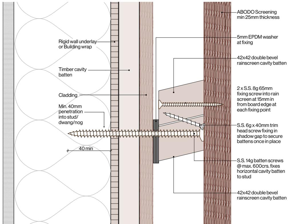
Abodo rain screen panelised cavity batten fix. Contact Abodo for further information.
