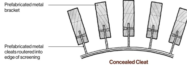
Cleat/bracket fixing – 32mm or greater timber thickness.
