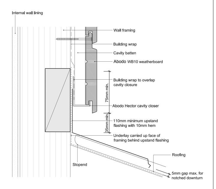
Note: refer to NZBC E2/AS1 Table 7 for apron flashing cover over roofing
