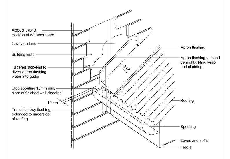
Note: refer to NZBC E2/AS1 Table 7 for apron flashing cover over roofing
